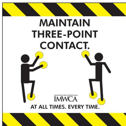
To prevent this scenario, employers should require employees to use the three points of contact when mounting and dismounting equipment. Many manufacturers now provide training videos on the specific procedure for three points of contact for different equipment.
